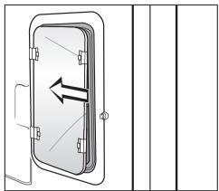
Push the glass cover back into the metal brackets with the cut out edge towards the rear.
